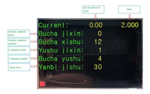
Note: The Hall current sensor has been calibrated before shipment, so calibration is generally not required;
