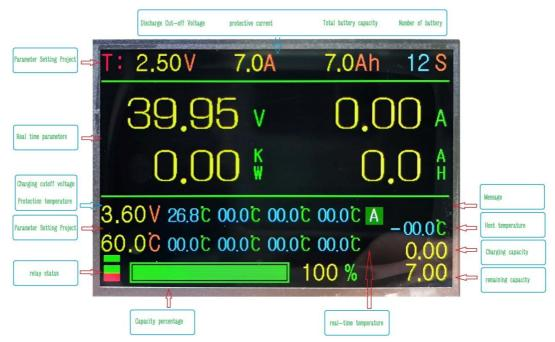
Note: The relay status is displayed in three sections, from top to bottom, which are pre-start relay, charging relay, and discharge relay. Green indicates open, and red indicates closed.
