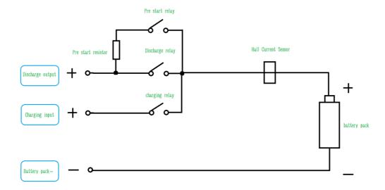
Note: For the same port connection method and split port connection method, the recommended pre start resistance value is 100 ohms, which can be calculated and adjusted based on the required pre start current, formula:Voltage (V)/Current( I)=Resistance Ohms, power above 100W, select power margin based on calculation;
